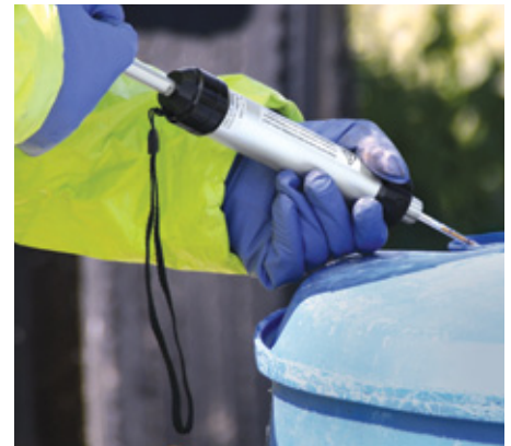
First responder uses RAE Systems colorimetric tubes and hand pump to measure VOC levels inside a barrel
