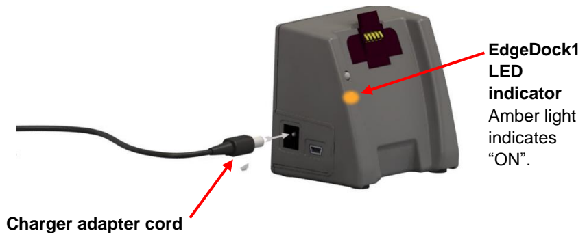
Figure 2-7 Attaching charger adapter to EdgeDock1 and EdgeDock5
