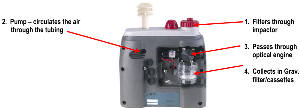
Figure 4-3: How the impactor functions
