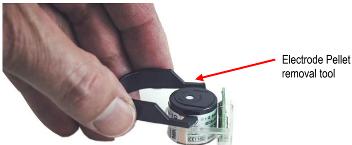
Figure 7-3: Removing the lamp with removal tool
