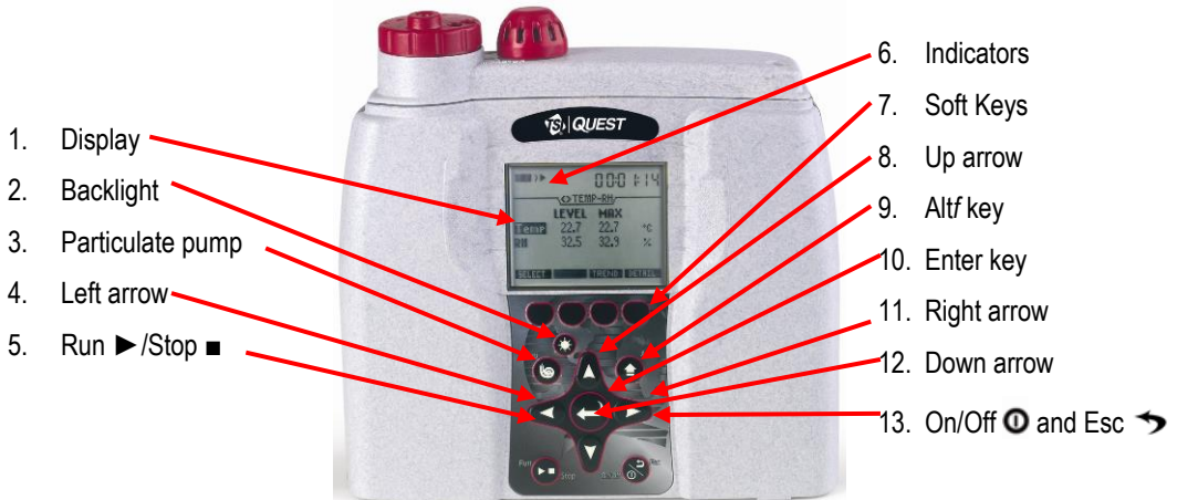
Figure 2-2: EVM keypad and display explained
