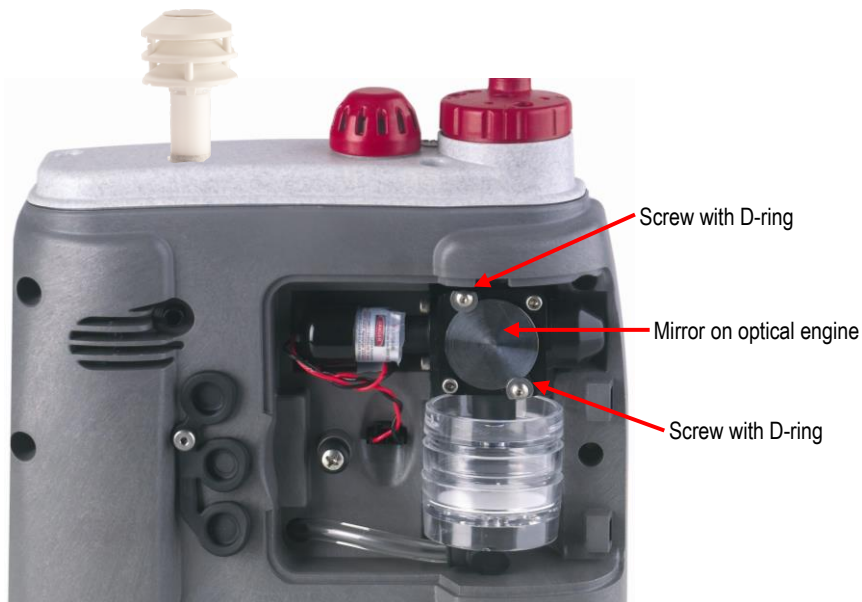
Figure 7-7: Optical engine and cleaning
