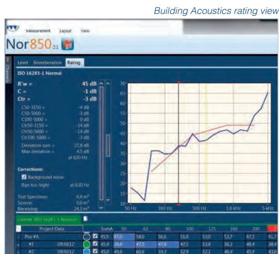
Building Acoustics rating view
