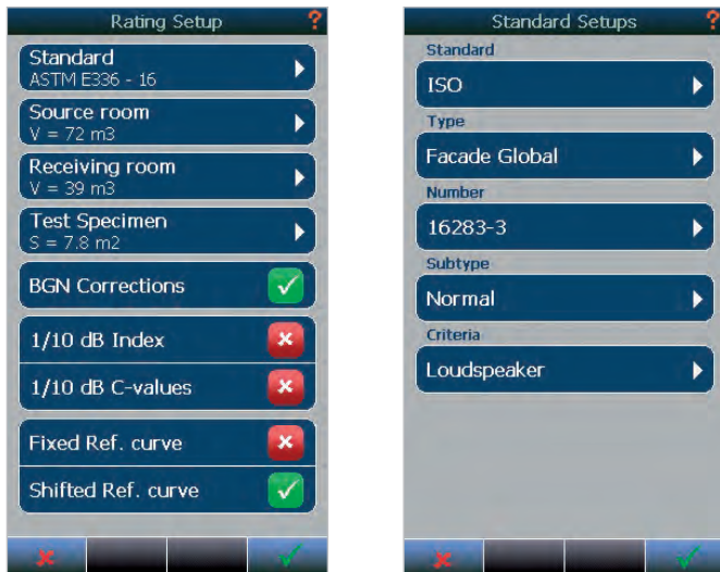
Setup menu for selecting standards. You may recalculate for additional standards based on already measured data.
