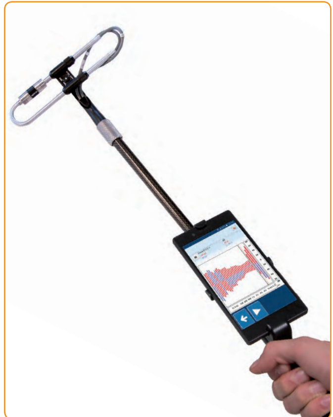
Other probe types may be used. The picture show B&K 2683 probe adapted to the Norsonic handle kit.
