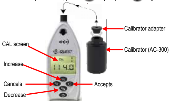
Figure 1-10: Calibrating the SD-200
