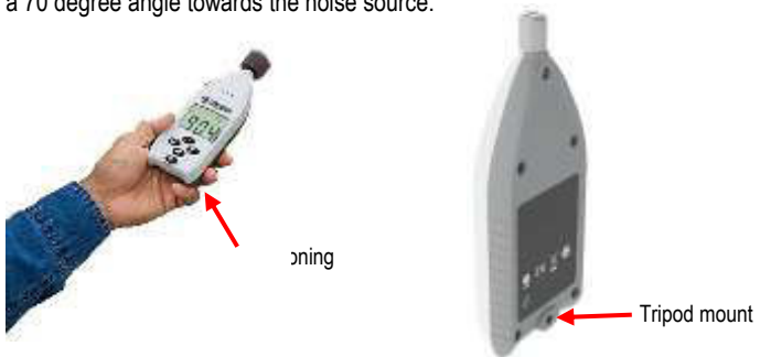
Figure 1-9: Positioning and tripod mount
